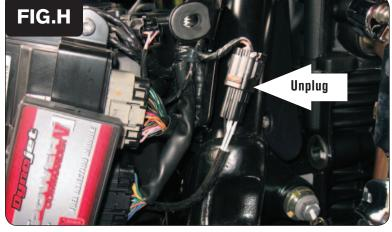
15 Unplug the stock O2 sensor from the main wiring harness.
